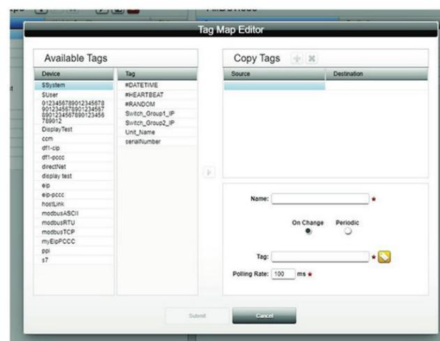
Figure 6: For each connected PLC, the Tag Map Editor enables each tag data source to be mapped to a data destination. The process is repeated for all connected devices. *Image source: Weidmüller*
