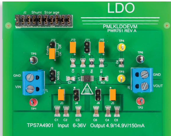
(a) TPS7A4901 LDO regulator under test
