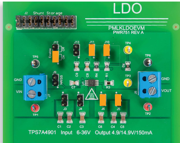
(a) TPS7A4901 LDO regulator under test
