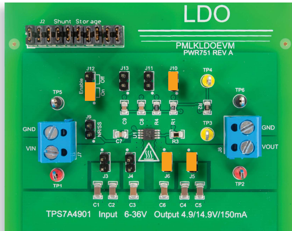
(a) TPS7A4901 LDO regulator under test
