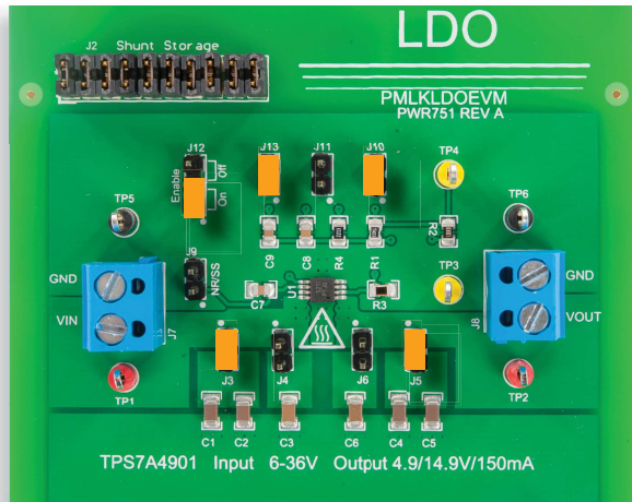
(a) TPS7A4901 LDO regulator under test
