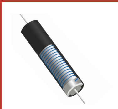
Figure 2: The fundamental construction of a wirewound resistor has changed little over time.
