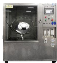
Rain test chamber
