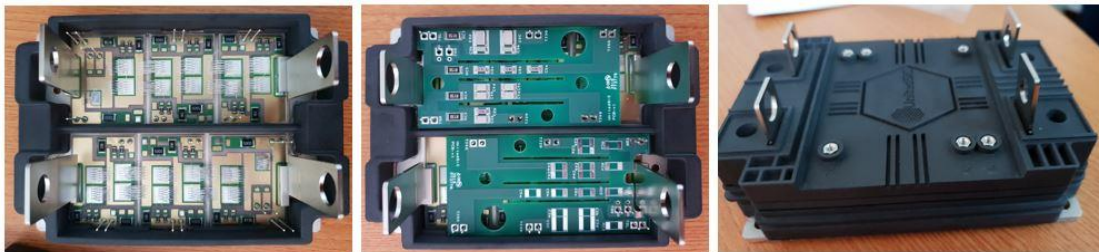
Figure 3: Internal structure of a 200A, 6500V Supercascode module under development. Power is largely dissipated in the SiC JFETs, which are on the DBC plane. The balance network goes on the PCB place since it does not dissipate much power.
